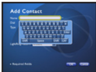
Step 4 • Add Contact: In the Name box, press "Keyboard" and use arrows to select letters or numbers.
